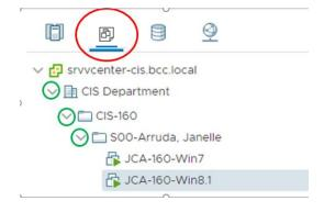
If your machine does not have a green triangle near it, it means the machine is not powered on.
